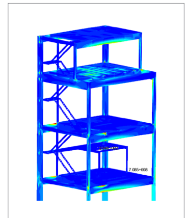
Figure 7. Von Mises stress tensor
